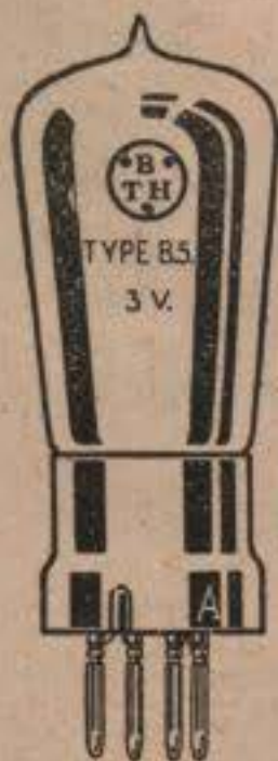
B5 Type Filament Volts - 2.5-3 volts Filament Current - 0.06 amps Anode Volts - 20-80 volts
